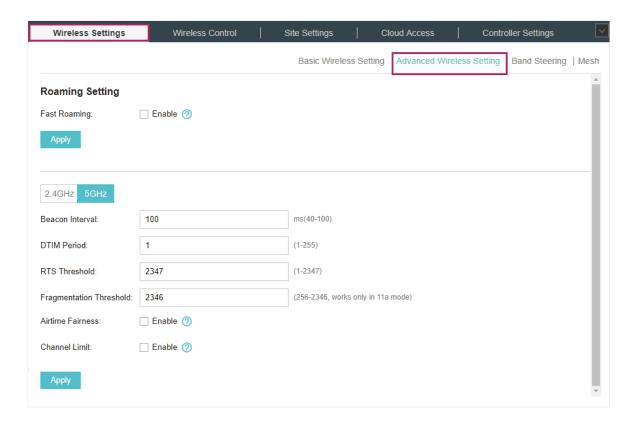
2. Enable Fast Roaming and configure the corresponding parameters.
