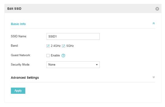
To make it easier for customers to connect, change the Security Mode from WPA-PSK to None. Customers can connect to the EAPs without password and be redirected to the Portal Authentication where the correct password will be required.
