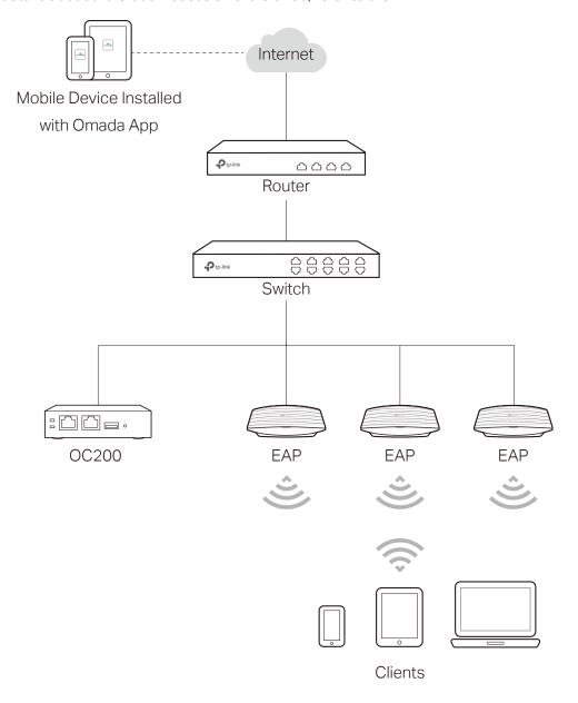
Follow the steps below to manage your network via Omada app in controller mode remotely. The following page is exampled with the iOS version of the app. The Android version is similar.
