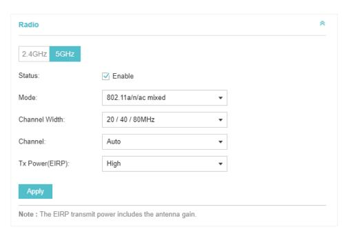
Select the frequency band (2.4GHz/5GHz) and configure the following parameters.
