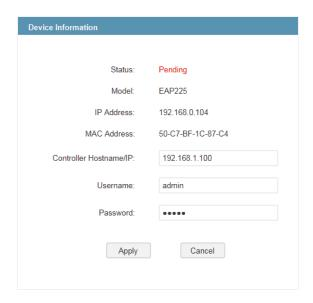
6. Click **Apply** to inform the EAP of the OC200's hostname or IP address. And then the connection can be established between the EAP and the OC200.
