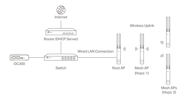
After all the EAPs are adopted, a mesh network is established. Then the EAPs connected to the network wirelessly also can broadcast SSIDs and relay network traffic to and from the network through the uplink AP.
